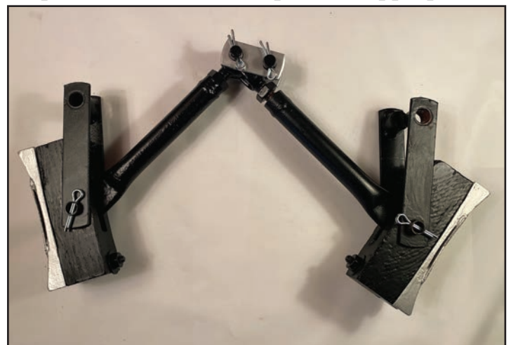
A nearly complete brake rehabilitation. These brakes will not only work well and are ready to bring your ride safely to a stop, but also look great when finished.
