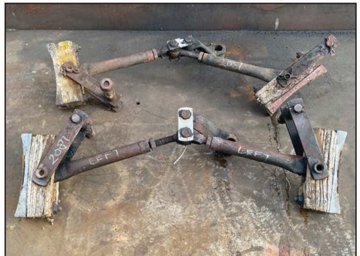
An example of a heavily corroded Fairmont M-19 brake assembly in need of rehabilitation
