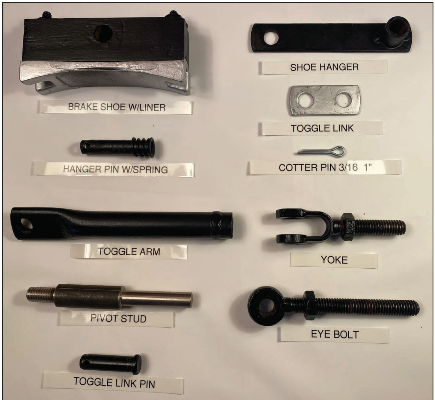
The primary components of a Fairmont brake assembly
